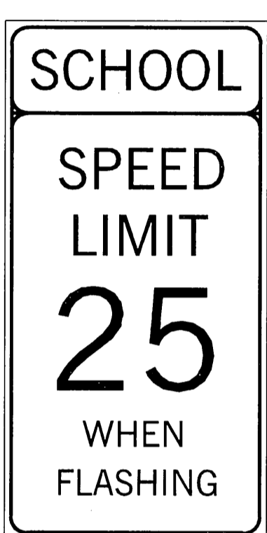
S5-1 SCHOOL SPEED LIMIT SIGN FOR DIMENSIONS SEE "STANDARD HIGHWAY SIGNS", LATEST REVISIONS.
