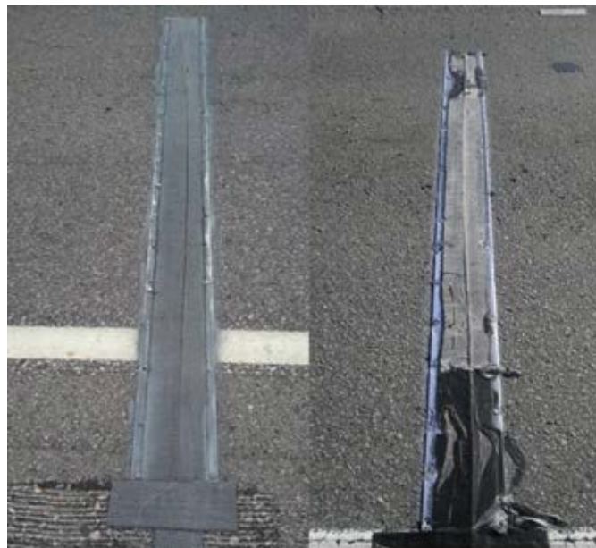
Figure 3.7 Deployment durability sensors after 20-day deployment and then after 40 days.
