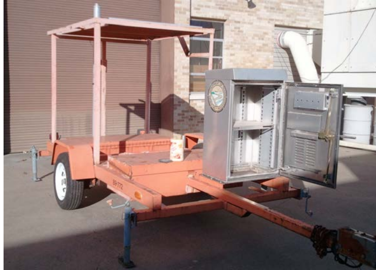
Figure 2.3 Portable WIM trailer before the installation of the power system, WIM controller and the REECE
