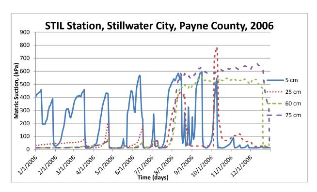
Figure B11. Matric Suction versus Time Plots For 2006.
