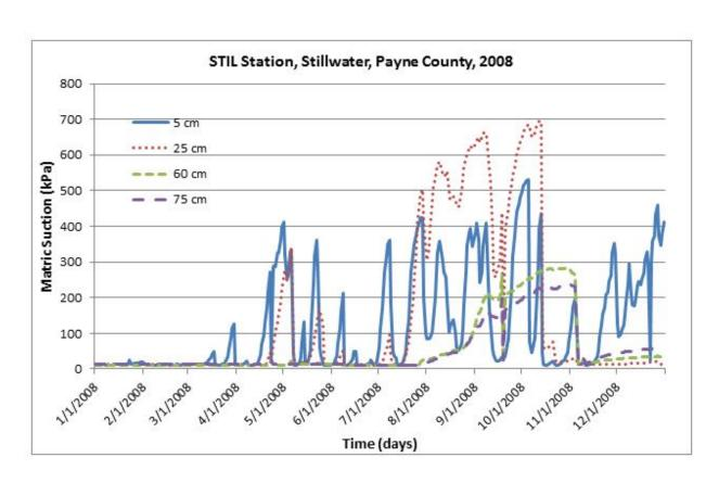
Figure 4.5. Matric Suction Variation with Time at Different Depths in Stillwater during 2008.
