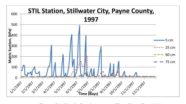
Figure B2. Matric Suction versus Time Plots For 1997.
