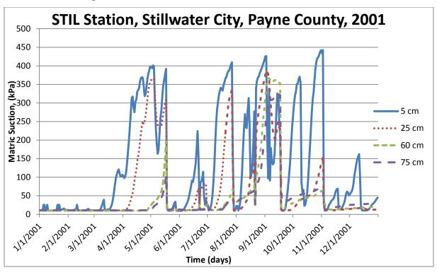
Figure B6. Matric Suction versus Time Plots For 2001.
