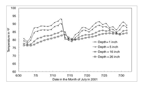
Figure 2.8. Typical Temperature-time Curves Predicted by EICM.
