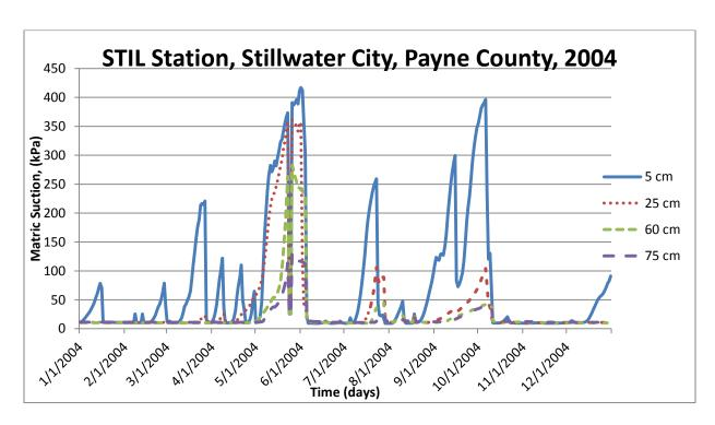
Figure B9. Matric Suction versus Time Plots For 2004.
