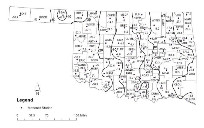
Figure 3.2. TMI Contour Map Based on Thornthwaite and Mather (1955) Equation.
