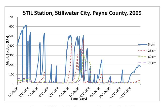
Figure B14. Matric Suction versus Time Plots For 2009.
