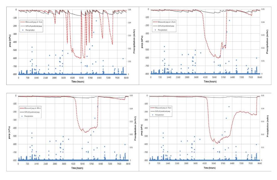
Figure 6.10. Measured and Predicted Pore Water Pressures at the WAUR Station.
