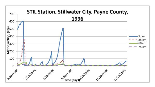
Figure B1. Matric Suction versus Time Plots For 1996.
