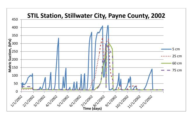
Figure B7. Matric Suction versus Time Plots For 2002.
