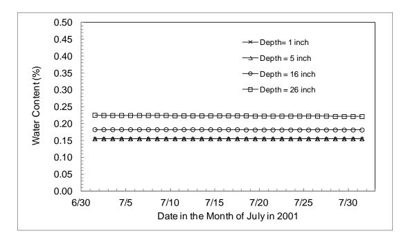
Figure 2.9. Typical Water Content-Time Curves Predicted by EICM.
