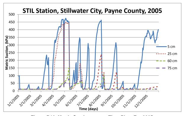
Figure B10. Matric Suction versus Time Plots For 2005.
