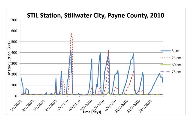
Figure B15. Matric Suction versus Time Plots For 2010.
