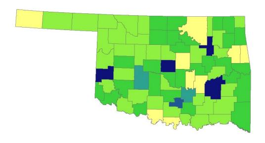
Figure 5.10. Six Soil Regions at 3 cm (K-means clustering).
