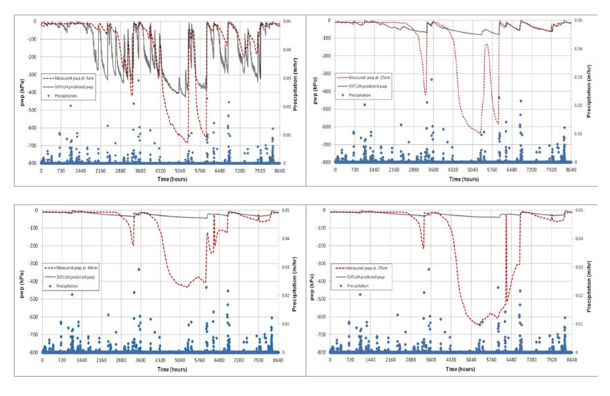
Figure 6.11. Measured and Predicted and Pore Water Pressures at the WIST Station.
