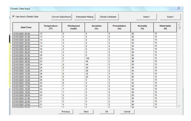
Figure 2.7. Typical EICM 3.4 Climate Data Input File.
