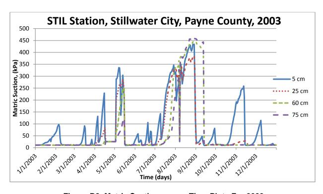
Figure B8. Matric Suction versus Time Plots For 2003.
