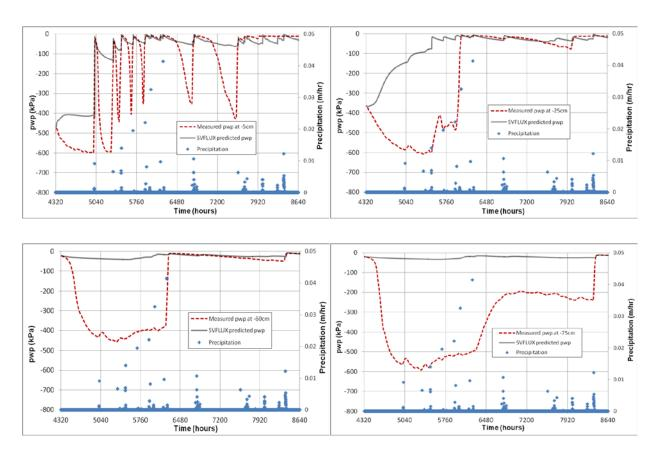
Figure 6.13. Measured and Predicted Pore Water Pressures at the WAUR Station with Initial Conditions at 4320 Hours.
