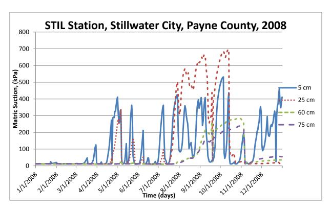
Figure B13. Matric Suction versus Time Plots For 2008.
