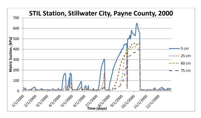
Figure B5. Matric Suction versus Time Plots For 2000.
