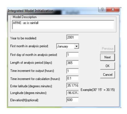
Figure 2.6. Typical Initial EICM Input Screen.
