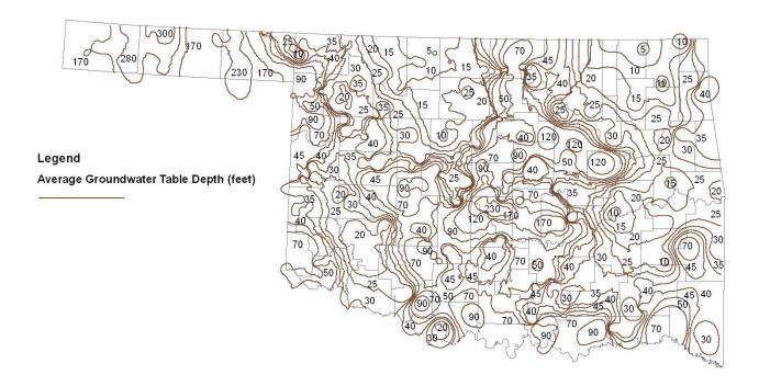
Figure 4.3. The Line Contour Map of GWT Depths in Feet.
