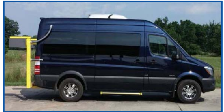
Figure 5. PaveVision 3D Ultra Laser Imaging Vehicle
