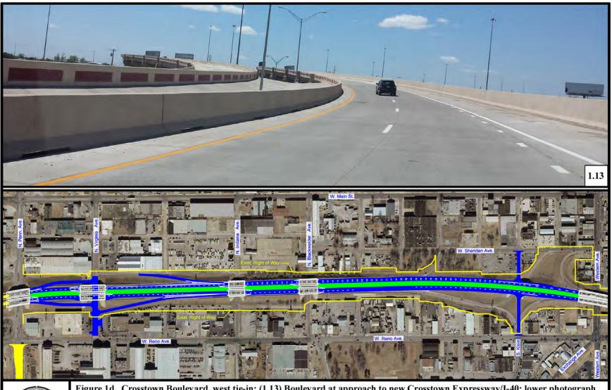
Figure 1d. Crosstown Boulevard, west tie-in: (1.13) Boulevard at approach to new Crosstown Expressway/I-40; lower photograph of aerial image illustrating existing right-of-way (yellow lines), at-grade roadway (blue and green), and elevated roadway (white) portions of Boulevard.
