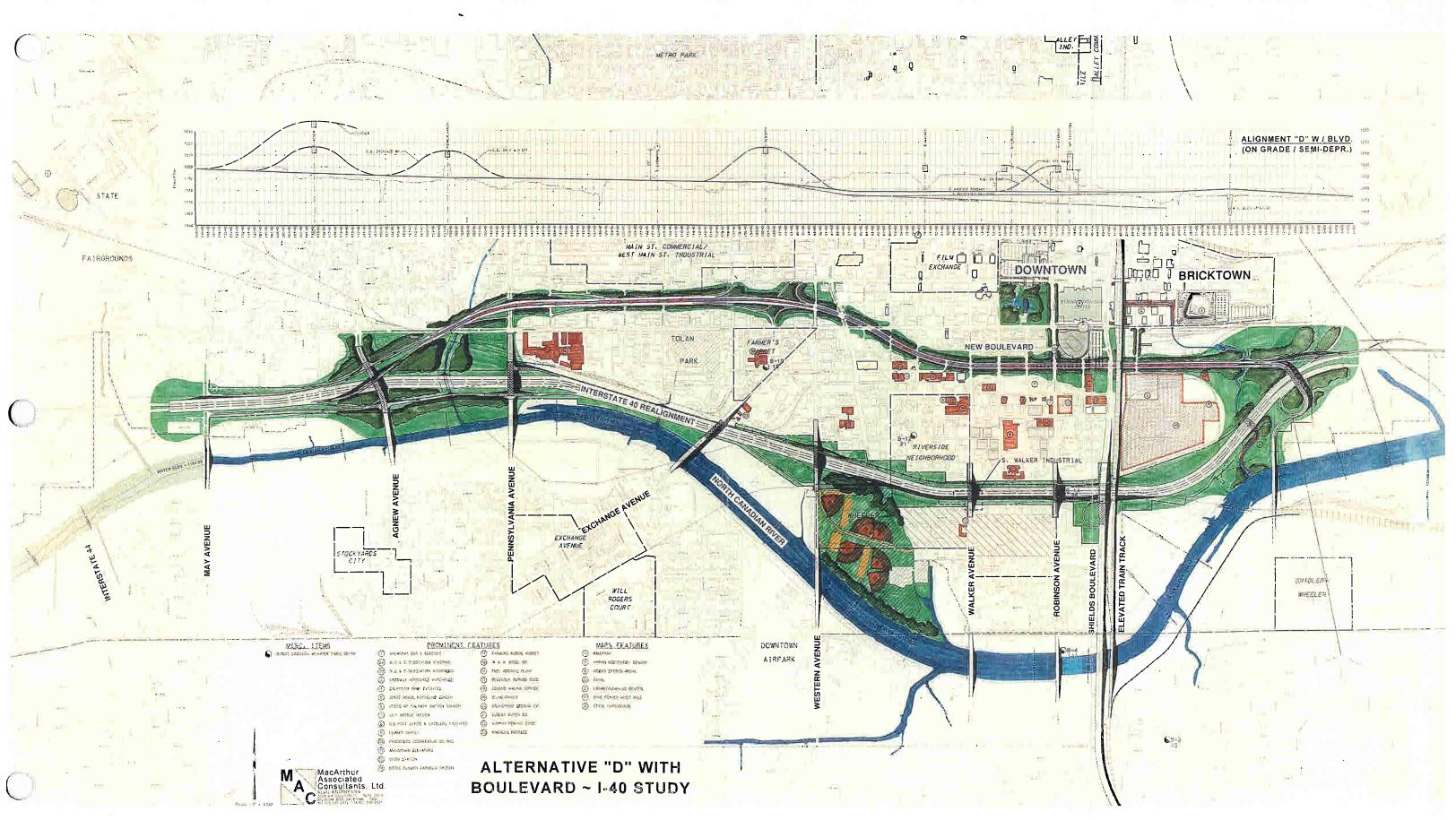
Alternative D from the EIS illustrating proposed Boulevard underpass under the elevated train track.
