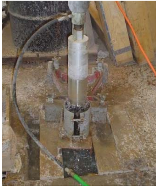
Figure 4 Sample being cored to required test diameter.
