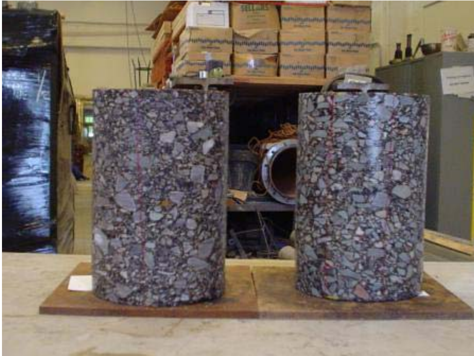
Figure 6 Test specimens for dynamic modulus testing.
