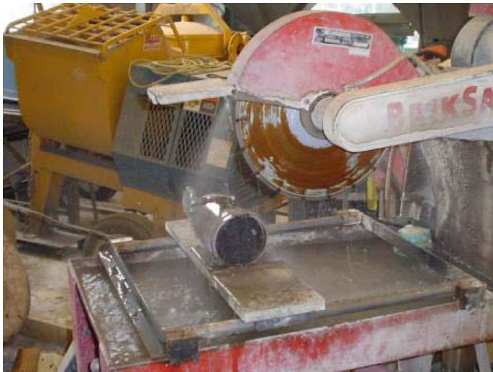
Figure 5 Sample being sawed to obtain parallel faces.
