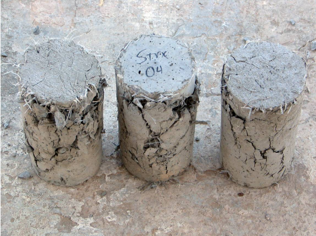
Figure 30: Fiber-reinforced concrete compression failure: ductile (Strux 90/40 10lb dosage)
