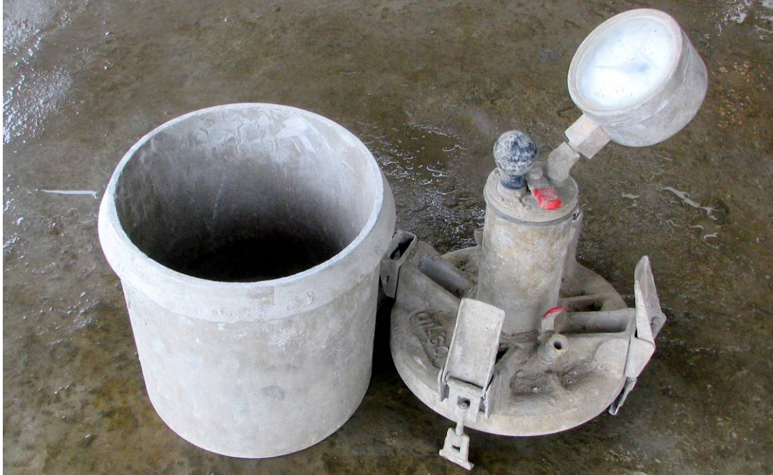
Figure 15: Air content pressurized air pot apparatus
