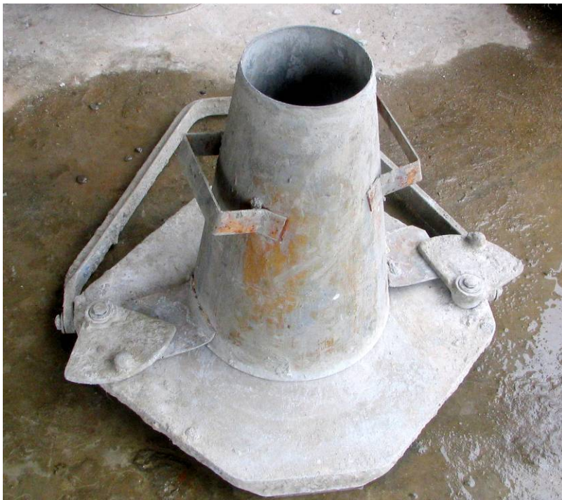
Figure 16: Slump test apparatus
