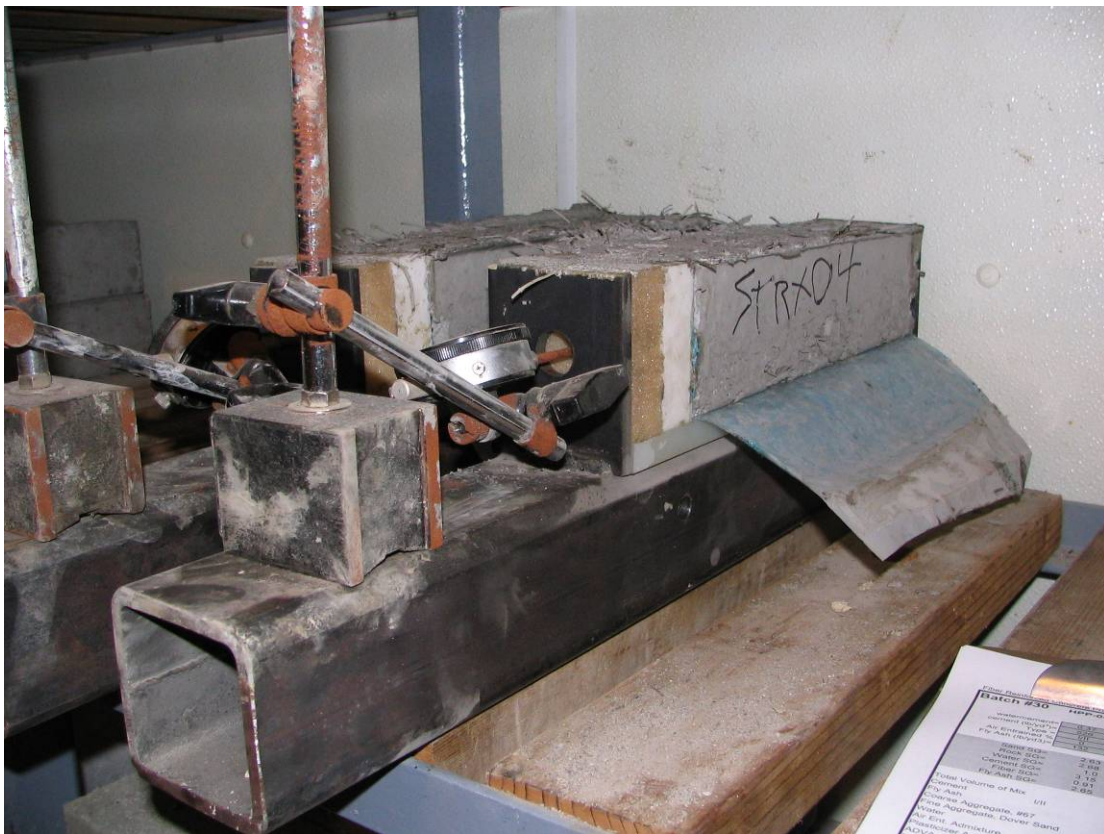
Figure 20: Unrestrained shrinkage from time zero test in progress
