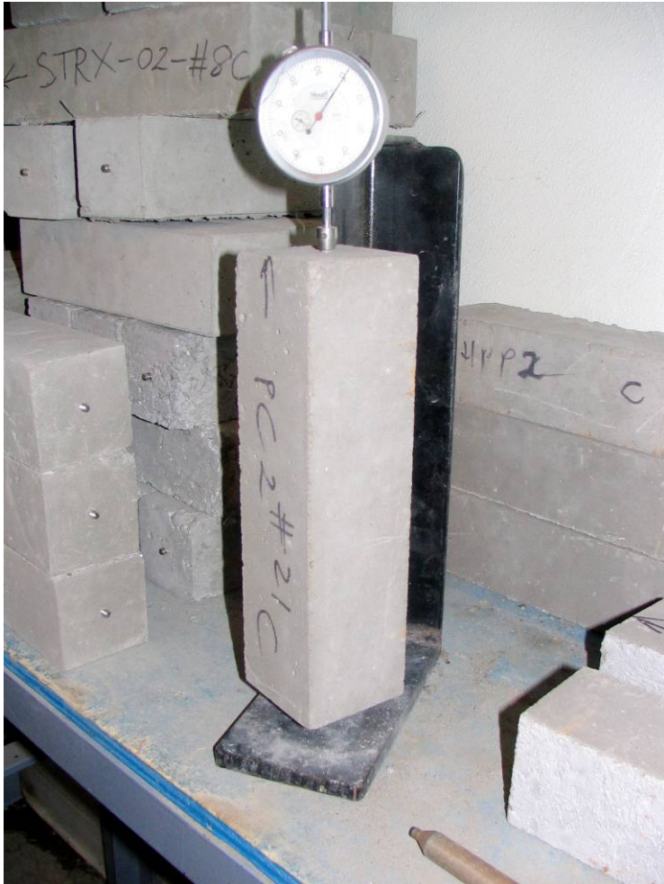
Figure 19: Unrestrained shrinkage test
