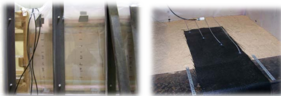
Figure 2. (a) A side view of the pullout test box filled with soil, (b) A PP woven geotextile instrumented with wire-line extensometers and placed at the middle of the pullout box.
