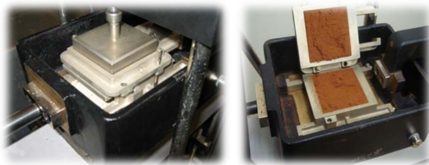
Figure 4. (a) Direct shear test cell before test, (b) direct shear test cell after test.
