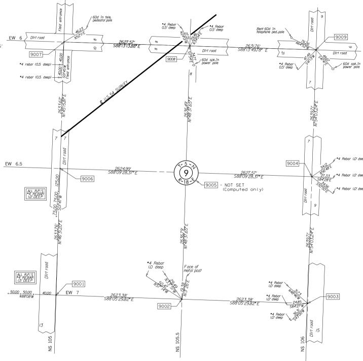
S 1/4 corner of section 9, T–5–N, R–18–E, C.M. ODOT Mon. no. T–70–390 Set #4 Rebar with cap stamped PLS1444 by single proportion between Gunnings filed corner one half mile west and found #5 rebar one half mile east.
