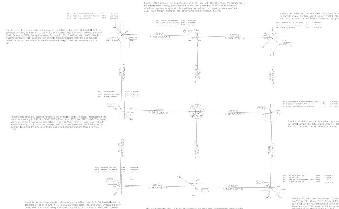
Found fences, structures, assorted references and centerline control for SH58. I reestablished the centerline according to SAP No. 775(2) SH58 Plans, dated 1951 and ODOT SW01704 Survey, Caddo County for SH58, Survey Completed February 2, 1951. Therefore 1 set a MAG Nail with washer according to said plans and surveys. Said monument agrees with the local evidence, therefore I accepted the monument for the corner and assigned it ODOT Monument No. C–8– 1204.
