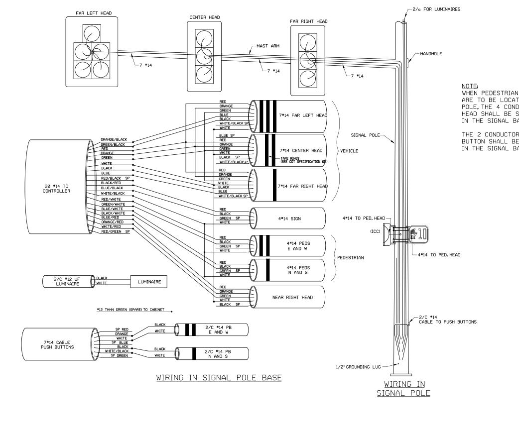
WHEN PEDESTRIAN HEADS AND PUSH BUTTONS ARE TO BE LOCATED ON SEPERATE PEDESTAL POLE, THE 4 CONDUCTOR FOR THE PEDESTRIAN HEAD SHALL BE SPLICED TO THE 20 CONDUCTOR IN THE SIGNAL BASE AND RAN TO THE PEDESTAL
