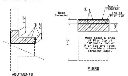
① Apply CIM 1000, Special Concrete Finish, to all surfaces shown with heavy lines and hatch (including Pedestal steps and ends of cap).
