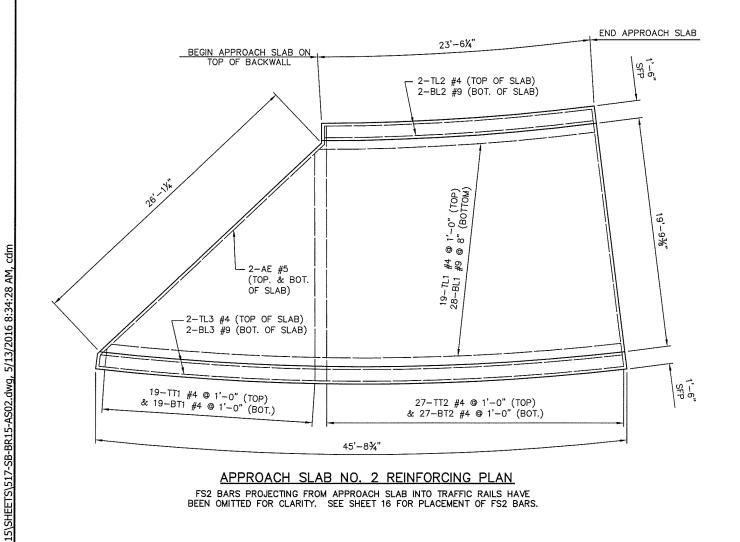
FS2 BARS PROJECTING FROM APPROACH SLAB INTO TRAFFIC RAILS HAVE BEEN OMITTED FOR CLARITY. SEE SHEET 16 FOR PLACEMENT OF FS2 BARS.
