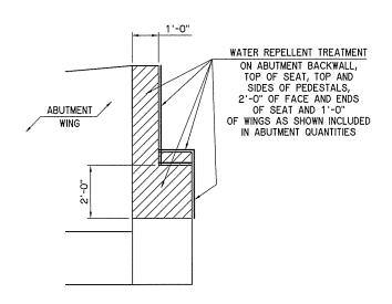
ABUTMENT NO. 2 WATER REPELLENT TREATMENT DETAIL
