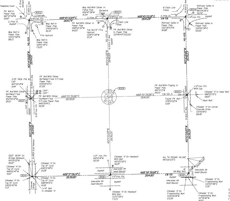
1/4 Section Corner — O.D.O.T. R—66—1074 — Found 1/2" Iron Pin with cap as referenced by Darren M. Smith RPLS #1552, May 28, 2010. No corner references were found. Established three more references in addition to the found PK nail also referenced by Mr. Smith. Also found and rejected a PK nail just 0.59' west of corner.
