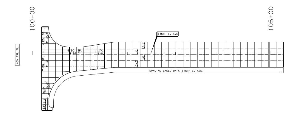
1. TRANSVERSE JOINT SPACING SHALL BE A MINIMUM OF TWO (2) FEET AND A MAXIMUM OF FIFTEEN (15) FEET, UNLESS SPECIFIED OTHERWISE.
