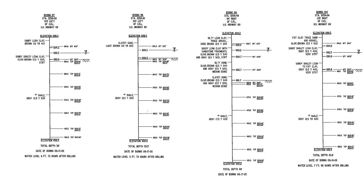
WATER ELEVATIONS SHOWN WERE OBTAINED AT THE TIME BORINGS WERE DRILLED AND MAY FLUCTUATE THROUGHOUT THE YEAR
