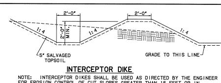
NOTE: INTERCEPTOR DIKES SHALL BE USED AS DIRECTED BY THE ENGINEER FOR EROSION CONTROL OF CUT SLOPES GREATER THAN 15 FEET OR IN LOCATIONS DEEMED NECESSARY TO RELIEVE SLOPE EROSION.
