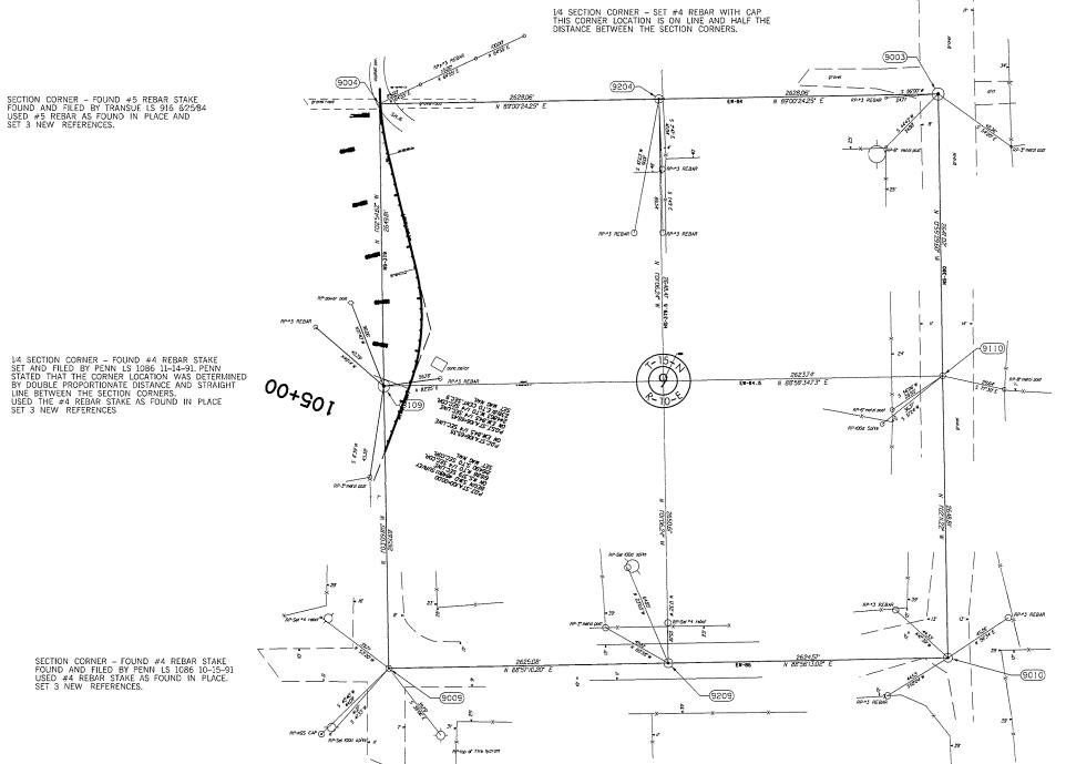
1/4 SECTION CORNER - FOUND #4 REBAR STAKE SET AND FILED BY PENN LS 1086 11-14-91 USED #4 REBAR STAKE AS FOUND IN PLACE. SET 2 NEW REFERENCES. SECTION CORNER – FOUND #5 REBAR STAKE FOUND AND FILED BY TRANSUE LS 916 62584 USED #5 REBAR AS FOUND IN PLACE AND SET 3 NEW REFERENCES.
