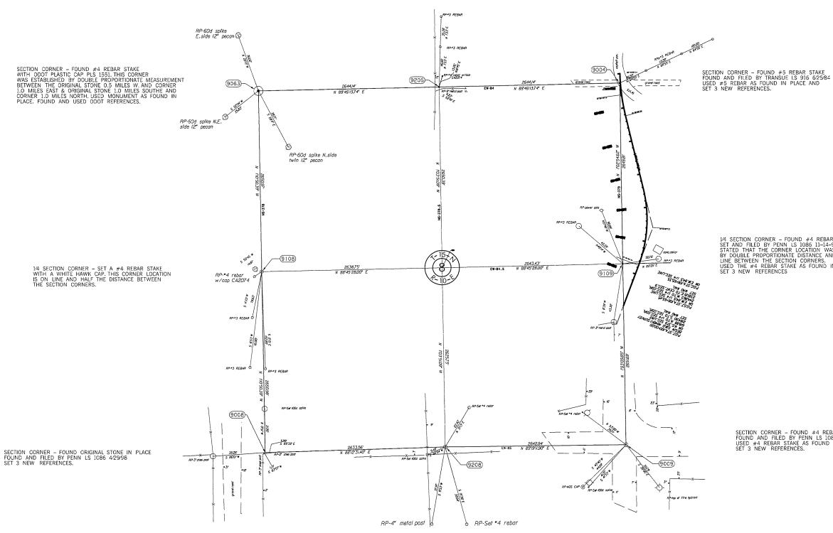
1/4 SECTION CORNER - FOUND #4 REBAR STAKE SET AND FILED BY PENN LS 1086 11-14-91. PENN STATED THAT THE CORNER LOCATION WAS DETERMINED BY DOUBLE PROPORTIONATE DISTANCE AND STRAIGHT LINE BETWEEN THE SECTION CORNERS. USED THE #4 REBAR STAKE AS FOUND IN PLACE SET 3 NEW REFERENCES
