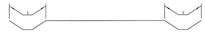
EROSION CONTROL TYPICAL SECTION 1 - SOLID SLAB SODDING VEGETATIVE MULCHING WILL BE USED FOR TEMPORARY EROSION CONTROL
