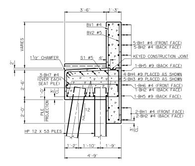
TYPICAL SECTION THRU ABUTMENT
