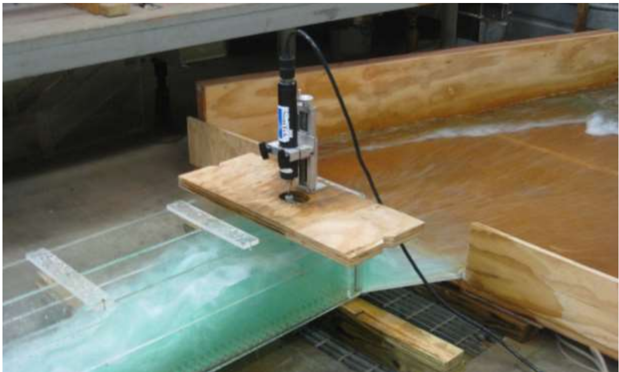
Figure 17. ADV Mounted over Flume
