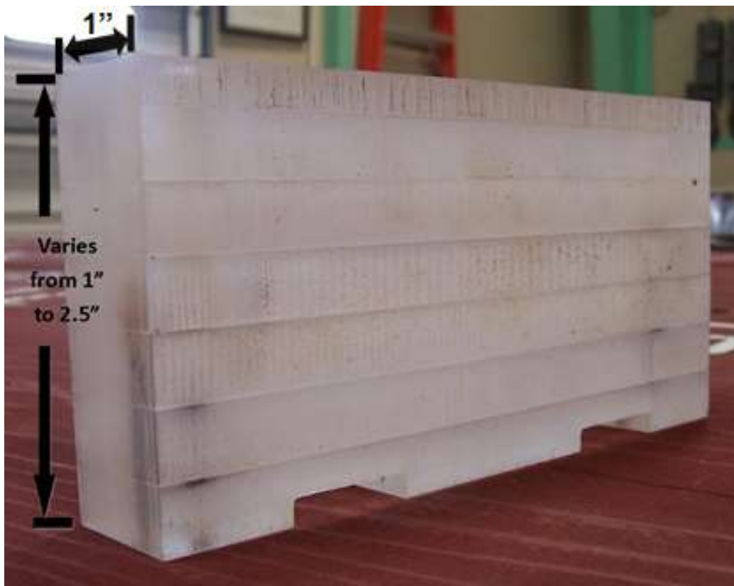
Figure 11. Typical sill dimensions
