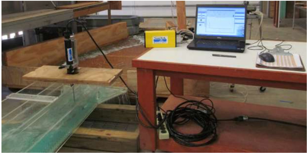
Figure 16. ADV plugged to measure the downstream velocity ( V_{d/s} )
